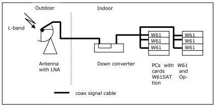
The monitoring system consists of three main components:
