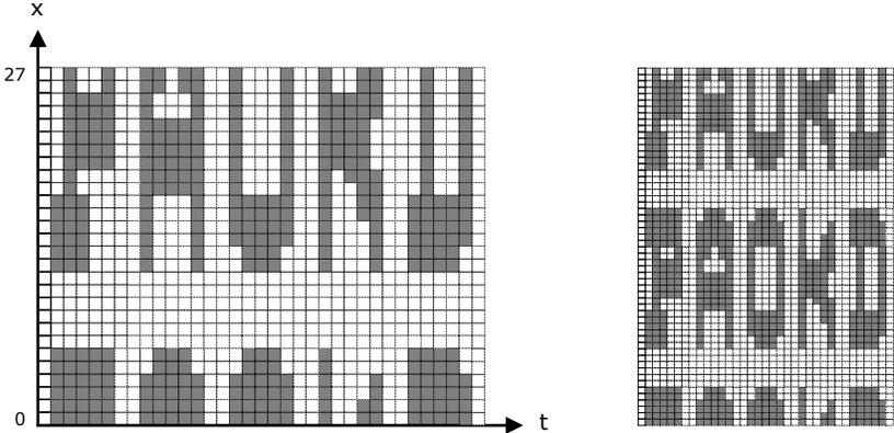
As shown on the left side of the image above, the message text will be cut and shifted. There is no synchronization marker in the FELD-HELL or FM-HELL radio signal, thus it is not possible to avoid this problem while decoding the signal. The easiest solution is to show the image twice, one below the other, as shown on the right side of the image.
