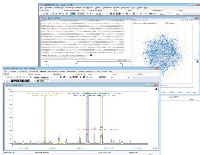
Simultaneous dual channel decoding on one W74PC card: STANAG4285 on AF#4 (instance 1) and SAT signals on IF70#1 (instance 2)
