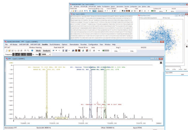
Simultaneous dual channel decoding on one W74PC card: STANAG4285 on AF#4 (instance 1) and SAT signals on IF70#1 (instance 2)
