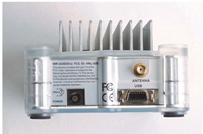
Fig. 20 and Fig. 21: The receiver. There is only one antenna plug (SMA) and the cooling ribs are cooled by a relatively quiet ventilator so they do not even become lukewarm. Excelsior is available from SSB-Electronic at 4,599 Euro ( www.ssb.de ).
