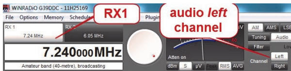
Fig. 5a and 5b: RX1 is tuned to a “good” frequency, here 7240 kHz, and the audio signal is sent to the left audio channel. RX2 is then tuned to a parallel frequency, which is sent to the right audio channel.
