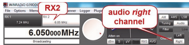
Fig. 5a and 5b: RX1 is tuned to a “good” frequency, here 7240 kHz, and the audio signal is sent to the left audio channel. RX2 is then tuned to a parallel frequency, which is sent to the right audio channel.
